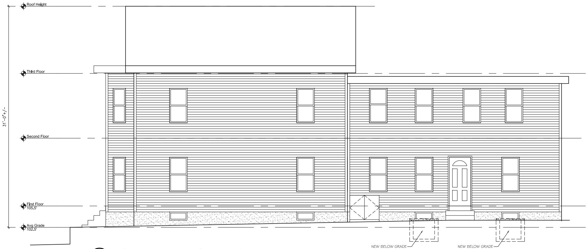
3 SOUTH ELEVATION - EXISTING Scale: 1/4" = 1'-0"
